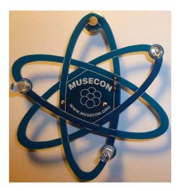
The heart of this blinkie is a tiny chip embedded in each of the three LEDs. When power is applied, the chip tells the LED to turn on and off.
