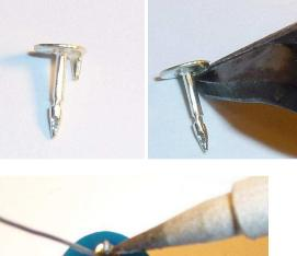
5. Flip the board over and insert the battery holder. Remember, orientation is important for the battery holder. Make sure the battery holder matches the printed outline. Flip the board over to the MUSECON side. Solder the battery holder.
